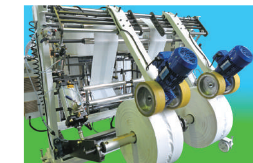
Inverter-motor tension control for jumbo film roll (The jumbo film roll is driven by inverter-motor, the speed can be synchronized with the main machine's speed.)
